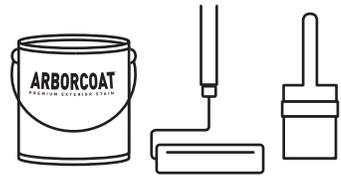
**4 Stain the wood.** Roll stain on the deck the full length of 2-3 boards at a time. Back brush to ensure proper coverage.
